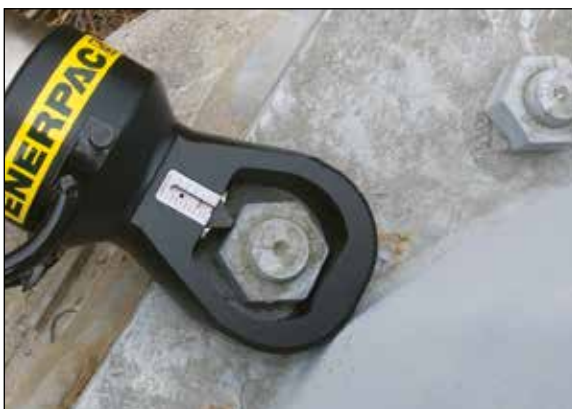
Nut splitter set for joint separation during inspection, maintenance and decommissioning operations. ▶
