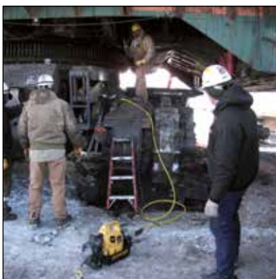
◀ Any brand of hydraulic torque wrench can be powered by the portable ZU4T-Series torque wrench pump.
