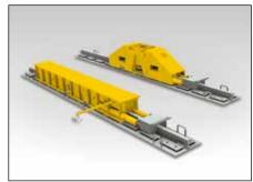
**HSK, HSKLH-SERIES, SKIDDING SYSTEMS**A system comprised of a series of skid-shoes powered by hydraulic push-pull cylinders, traveling over a pre-constructed track.
