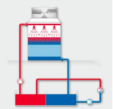
Cooling circuit with a conventional open cooling tower
