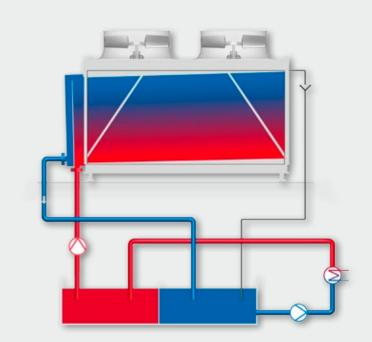
Cooling circuit with a semi-open hybrid dry cooler
