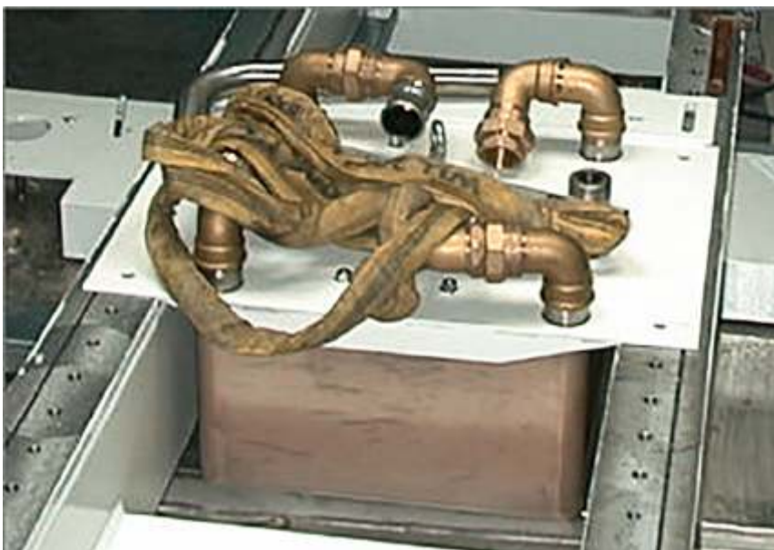
The B45x120 is mounted in a groove below the test equipment
