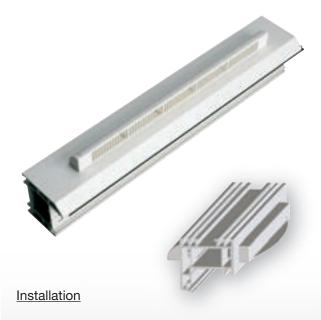
Controllable/Permanent: Routing: 12 mm x 310 mm Push fit to frame and push fit the buttons
