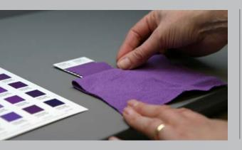
Colour requirements for manufacture and retail are complex and diverse. To ensure product colour, several types of light source are used (e.g. Artificial Daylight and a Point of Sale Light. Multiple light sources are also necessary to reveal colour inconsistencies and metamerism.
