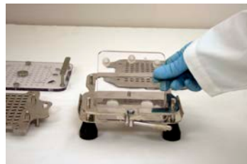
5. Lift out clear Spacer Plate and replace with new size Spacer Plate.
