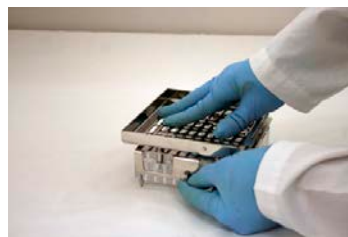
1. Unscrew 2 thumbscrews holding Orienter Tray to Base.
