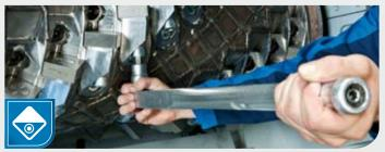
Monofix-System Knife mounting with one screw only; quick change of cutting knives
