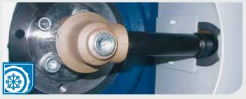
Rotor Cooling (optional) Constant surface temperature on the rotor using a closed cooling system
