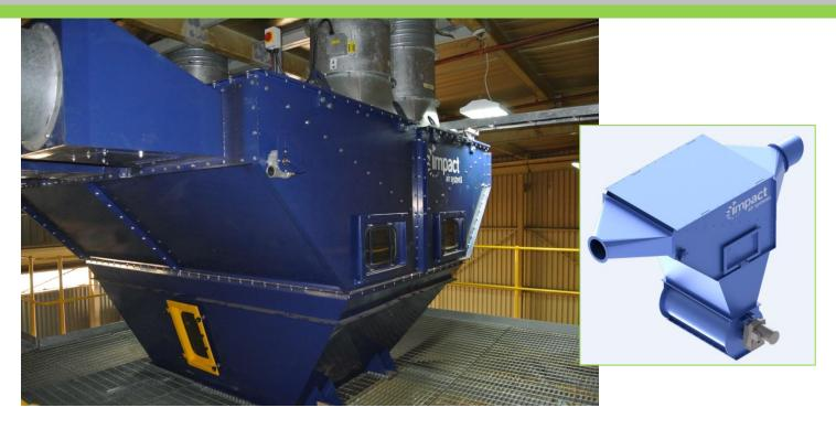
The separator's main function is to separate the waste material from the conveying air stream. The separator assembly consists of a perforated screen plate, inclined downwards at an angle inside metal housing.
