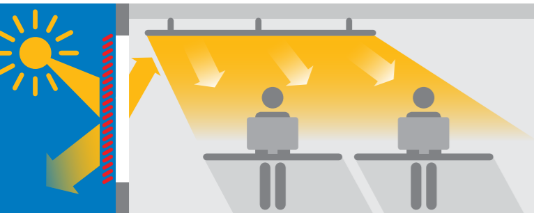
Daylight deflection into the heart of rooms using Atlantic Glow with active solar protection.
