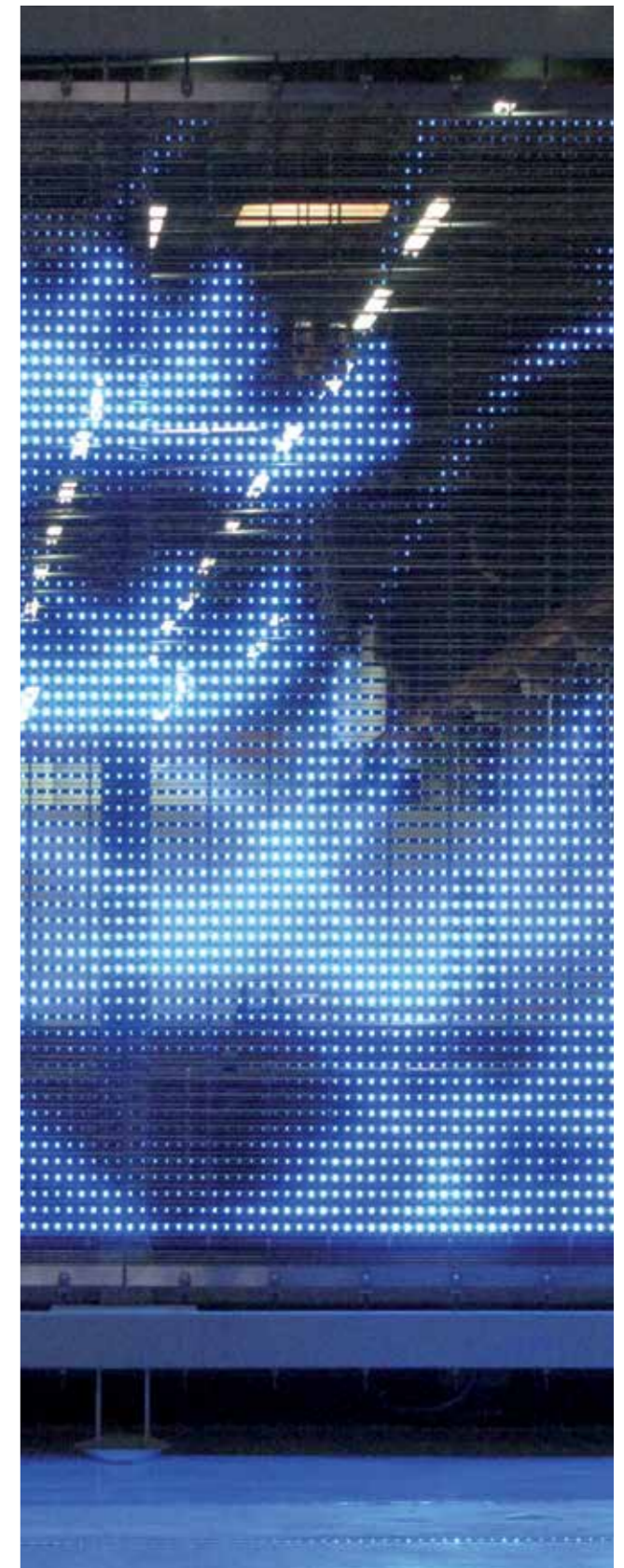
Mediamesh® SMD system - first prototype of the new SMD system (10)
