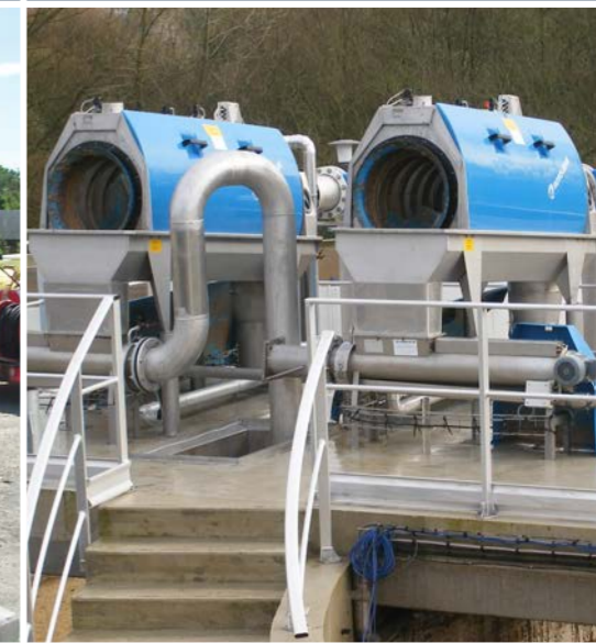
Roto-sieve Drum Screen and screenings handling equipment for liquid/solids separation ▲
