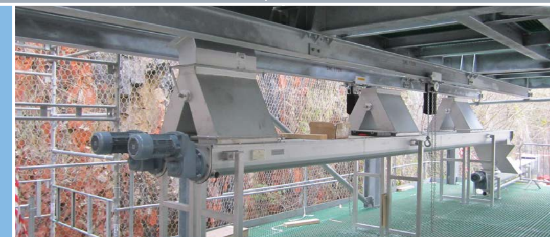
Shaftless screw conveyor installed at Buxton STW for Severn Trent Water ▼
