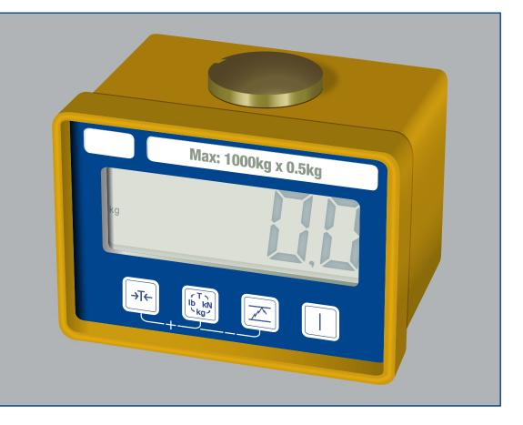
The Loadblock Plus is a low capacity, self-indicating compression load cell, used in many testing and load monitoring applications worldwide. The integral display eliminates the need for a separate display or cable assemble that can be easily damaged. Applications include the measurement of loads associated with the testing of hydraulic presses, cylinders or jacks.
