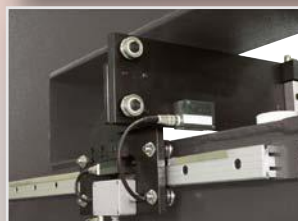
Distance measurement of X-and Y-traverse paths
