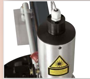
Cylinder prepared for installing a laser pointer
