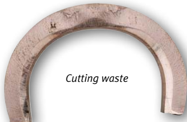
Image surface cross section; reworking (regrinding) by the customer recommended
