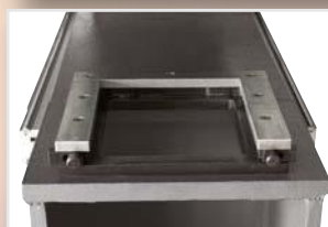
Die holder, tool exchange possible even with a mounted control cabinet door
