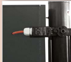
Electric safety locking for accident prevention.
