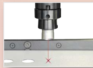
Laser pointer for optical indication of tool centre
