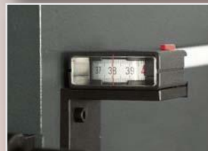
Measuring tape indicator for Y axis
