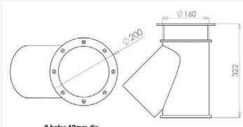
8 holes 10mm dia Mounting detail
