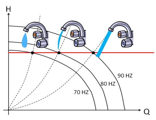
The control module receives the pressure signal from the pressure transducers and varies pump speed to maintain a constant set pressure regardless of water demand. In addition to the constant pressure control, CM can also the following control modes:
