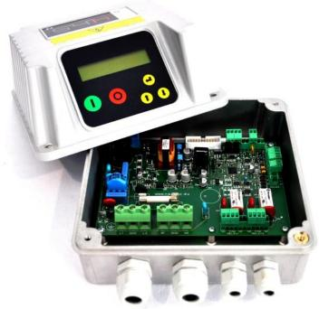
CM control module, mounted aboveground, manages the pump operation by changing pump speed to maintain the desired pressure in the system regardless of water demand.
