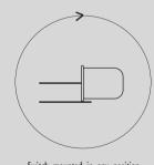
Switch mounted in any position.
