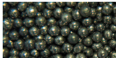
FIGURE 11-3A High Quality Shot Peening Media
