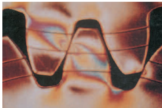
FIGURE 4-3 Polarized View of Applied Gear Stresses
