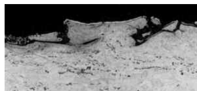
FIGURE 11-2A Damaged Surface from Broken Shot Media
