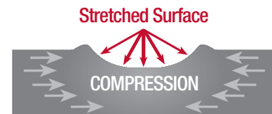
FIGURE 1-2 Compression Resists Fatigue Cracking
