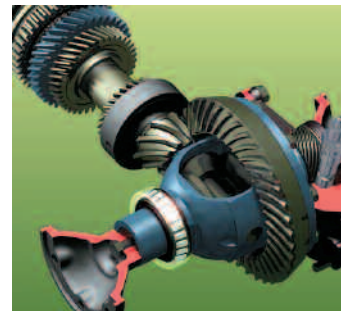
FIGURE 4-2 Ring and Pinion Gear Assembly
