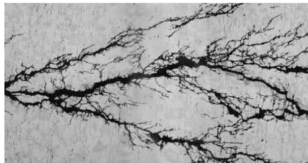
FIGURE 8-2 Stress Corrosion Cracking Failure of 300 Series Stainless Steel
