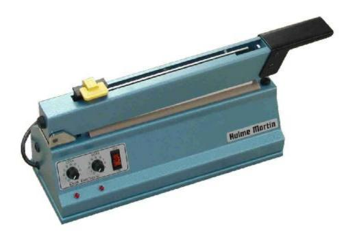
General purpose machines with many applications. Used extensively by hospitals, laboratories, retailers, engineering and other industries. This CD model has a dual electronic timer for complete control of the heating and cooling cycle and a cutter to facilitate bag production from lay flat tubing. This machine is simple to maintain with consumable spares being easy to fit and available from stock.
