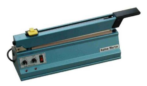
General purpose machines with many applications. Used extensively by hospitals, laboratories, retailers, engineering and other industries. This CD model has a dual electronic timer for complete control of the heating and cooling cycle and a cutter to facilitate bag production from lay flat tubing. The machine is simple to maintain with consumable spares being easy to fit and available from stock.
