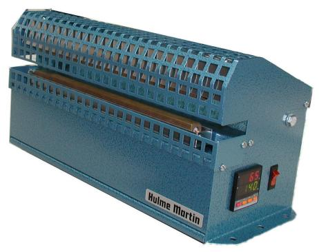
For high-integrity crimp seals on cellophane, polypropylene, heavy duty barrier foils, coated papers and other laminates. Both the upper and lower jaws are heated for use with heavier materials or gussetted bags. The machine's temperature is digitally controlled, with a thermal fuse fitted for excess temperature protection, this allows for consistent and easy temperature selection up to 180°C, which is lockable to prevent user intervention.
