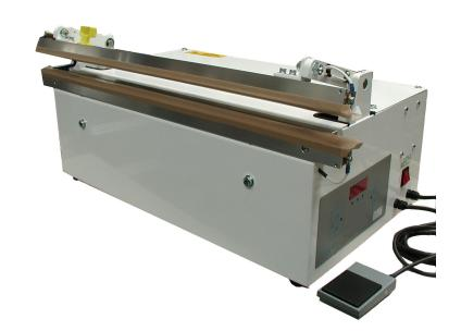
This unit is manufactured to enable 'lay flat' tubing to be welded without obstruction, a manual cutter is available to trim off excess material or produce bags from reels of material. NOTE machines fitted with a manual cutter produce a cut length 4 inches (100mm) less than the seal length.
