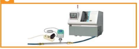
By means of quick couplings the flow sensor can be integrated quickly into the feed hose of a machine. During the shutdown of the machine it is possible to determine the leak rate, the actual flow can be obtained when the machine is running. The power supply is effected via the power socket by means of the mains unit. For data recording over a longer period of time we recommend to use the compressed air analyzer DS 400 mobile.
