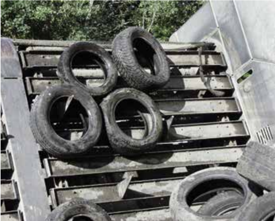
A hook lifter separates the whole tires for a controlled and continuous feeding.
