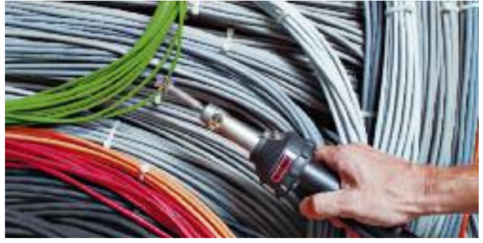
Fitting a solder shrink connection with the HOT JET S outfitted with a push-fit sieve reflector.
