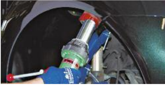
Accelerating the drying process of varnish, paint and body filler using the ELECTRON.
