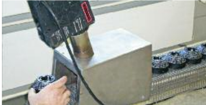
The HOTWIND S is perfectly suited for drying and firing of color on plastic components.
