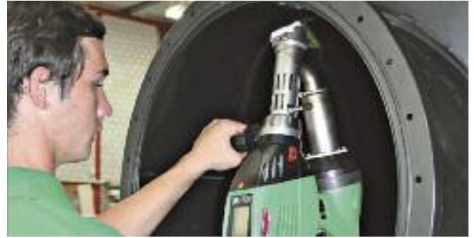
Even inside radiuses are easy to weld.
