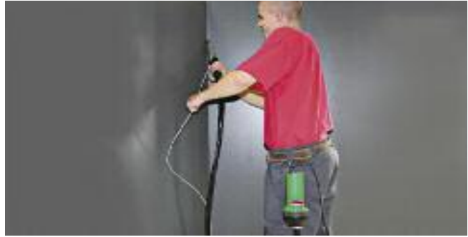
The MINOR blower as an air supply for the DIODE PID.
