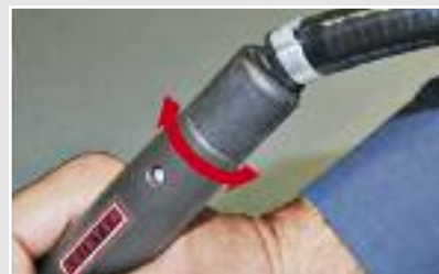
Swiveling air hose for easy working.
