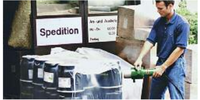
Flameless shrink-wrapping of pallets and bulky goods with the FORTE S3.
