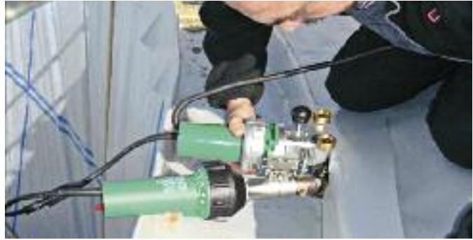
The TRIAC DRIVE PID allows even horizontal welding.
