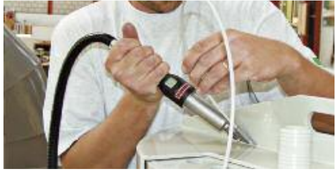
Draw welding using the compact and lightweight WELDING PEN R.
