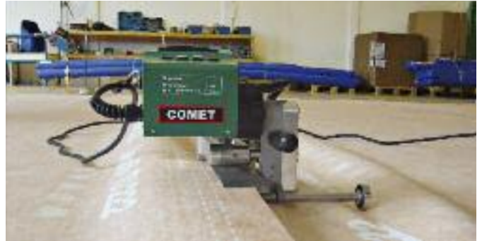
Hands-free welding due to integrated guiding plates.
