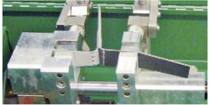
Testing a weld seam with the EXAMO USB.
