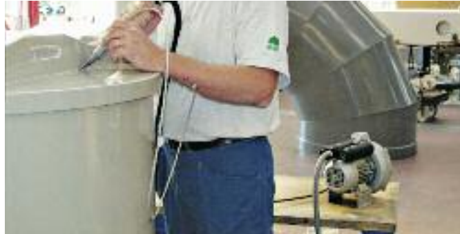
ROBUST blower, serving as the external air supply for the WELDING PEN.
