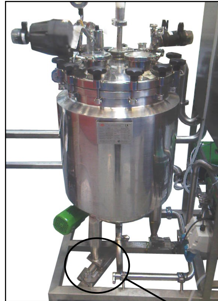
Solution Preparation Vessel
