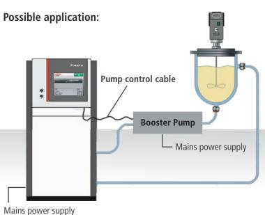
The Mag Drive Booster Pump can increase your fluid pressure up to 2.1 bar. The stainless steel design of the Pump provides excellent resistivity against chemical effects. The magnetically driven design guarantees 100% leakage free operation over an extraordinary temperature range of -90 ... +250°C.
