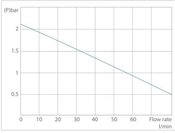
(measured with fluid with density of 1kg / dm³)
