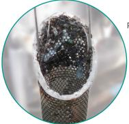
Pond strainers catch larger particulate but finer items pass through settling out in low velocity areas.
