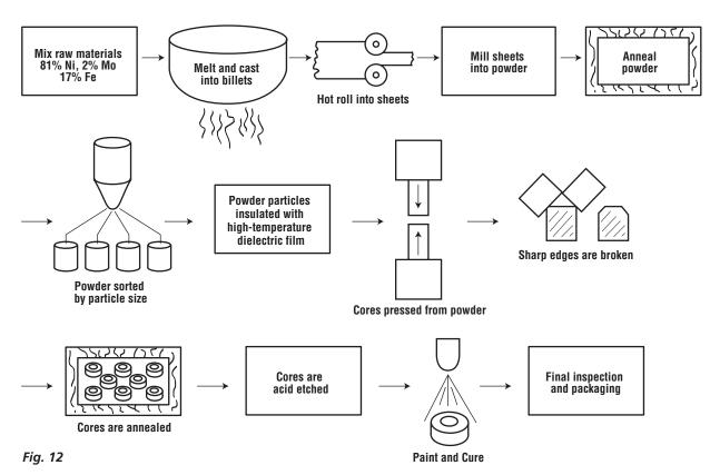
Another type of powder core manufactured by Arnold is the MPP core, pressed from powder made of 81% nickel, 2% molybdenum and 17% iron. We manufacture our own MPP powder from precisely controlled raw materials that are melted and cast into billets, which are hot-rolled into a brittle sheet. This sheet is then milled into powder form. Insulators are mixed into the MPP powder before pressing into cores at high
