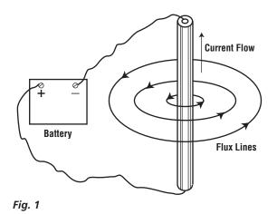
units and **AMP-turn per meter** in SI units. Units of MMF (magneto-motive force) are **Gilbert** in CGS and **AMP-turn** in SI systems.
