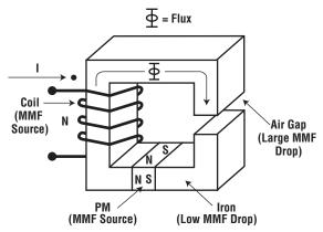
Fig. 6 Typical Magnetic Circuit
