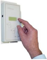
**1** - The user "wakes up" the Timy-USB badge Reader by pressing the only button on the device. Timy displays the time and is ready for an ID-badge.
