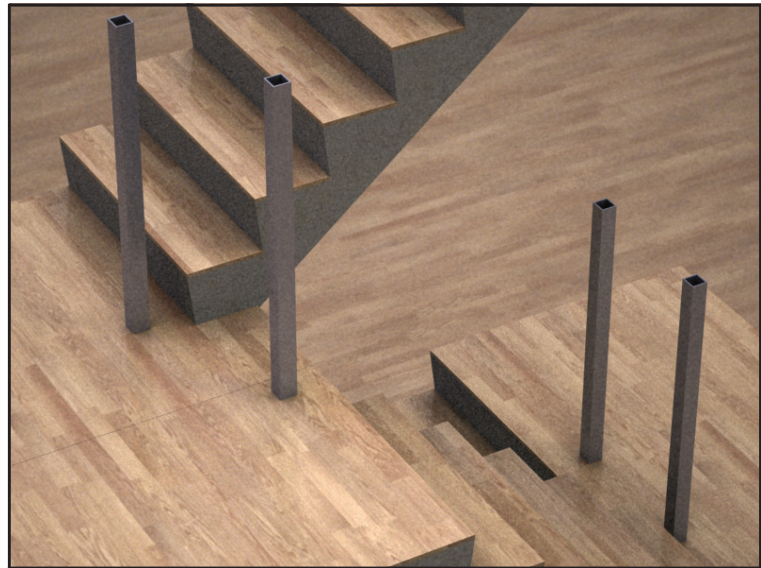
8 Finish the flooring, decking, screed, floor finish etc. to the required height. This should conceal the base plate and bolts
