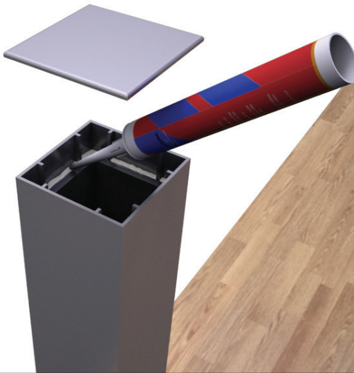
13 Inject an additional amount of silicone into the gaps between the steel post and cover post on the inside
