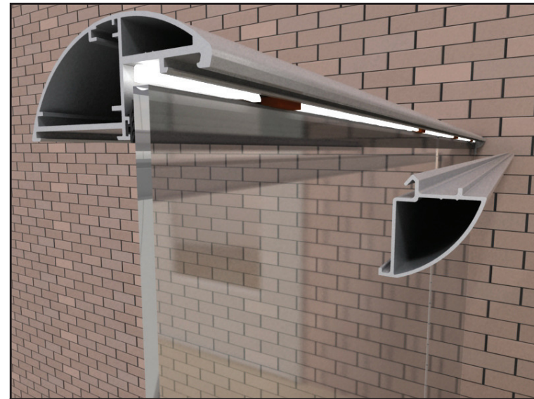
62 Replace the full length glazing beads
