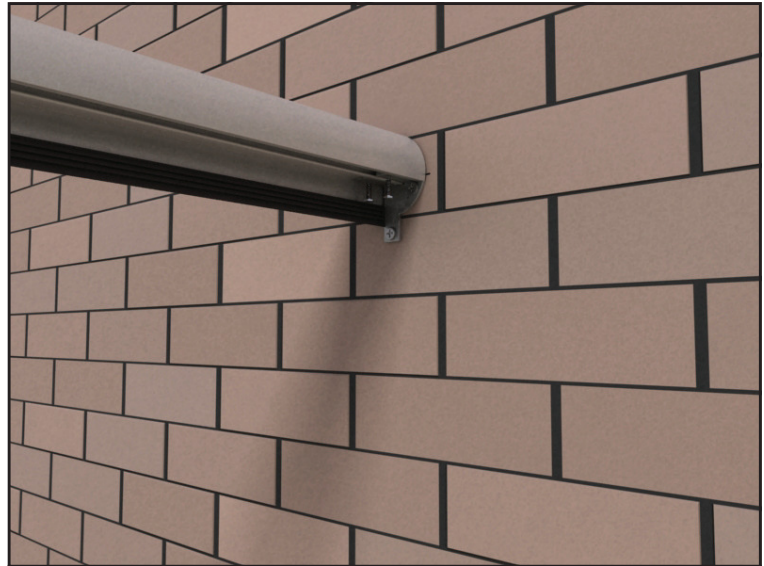
27 Drill 4mm holes through brackets in the handrail. Fix the handrail to the wall bracket using the No. 10 x 3/4" S/tapping screws
