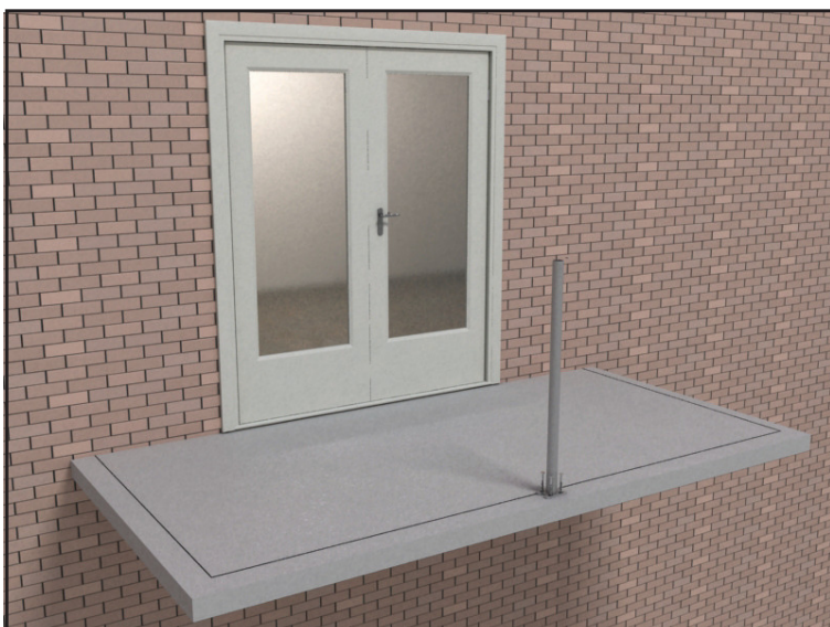
15 Position the primary steel post in the correct position
