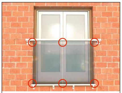
13. Line the glasses up in position so that they are spaced correctly between each other and the wall.
