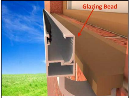
2. Line up bottom track vertically to allow access to the glazing bead from the inside.
