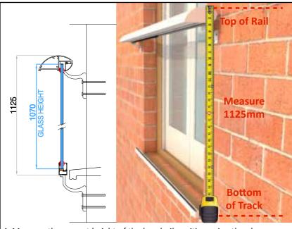
4. Measure the correct height of the handrail position using the above drawing. Do not scale from this drawing.
