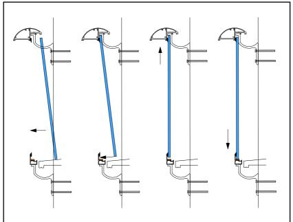
10. Follow these steps to insert the glass panels in position using the temporary glazing beads and rubber gaskets.
