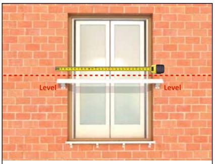
5. Centre the handrail to be central with window giving an equal overlap on both sides.
