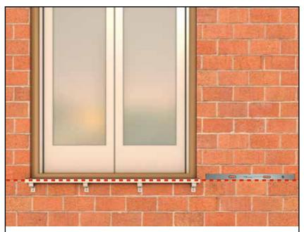
1. Line up bottom track to be level and central with the window opening.
