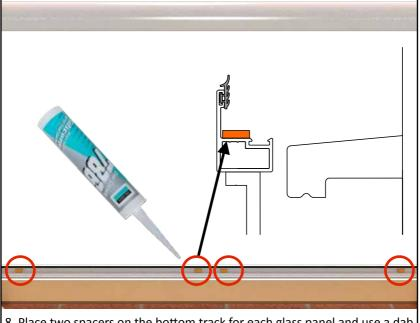
8. Place two spacers on the bottom track for each glass panel and use a dab of silicone to keep them in place.
