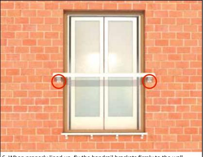
6. When properly lined up, fix the handrail brackets firmly to the wall.
