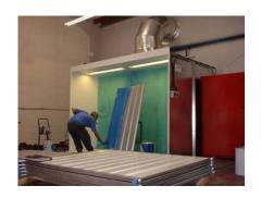
Dry Filter Spraybooths with centrifan, manometer and 'full face' extraction system
