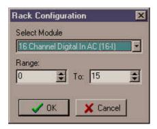
Select the new element form the drop down list, then enter the range (if required) in the boxes. The example above shows a 16 channel input card configured as I0 to I15.
