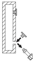
Immediately fit new plug. Tighten to 27-34 Nm and lock by disturbing cover material into the slot of the plug using a punch. For Plug Type A, it is recommended that the old plug is re-used with a new seal and the plug tightened to match existing peining marks.
