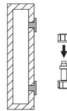
Fit cap nut to container and ensure both cap nuts are fully screwed on but not over-tightened. (Do not use spanners).
