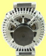
UNA2357 alternator Prone to diesel leaks.
