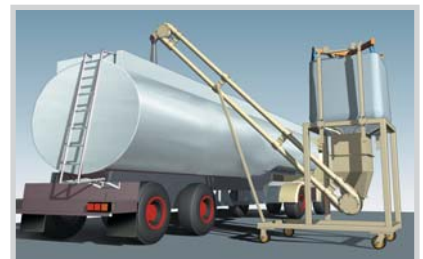
Bulk bag discharger and AMC loading road tanker.
