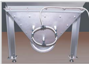
Inlet chute with aeration device.
