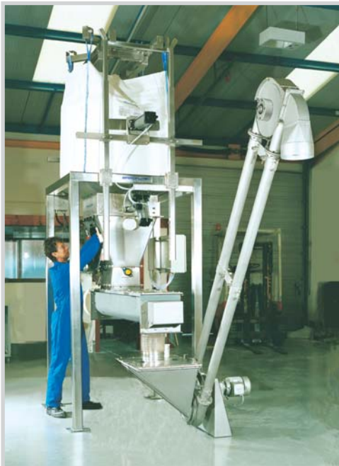
AMC designed for handling titanium dioxide. The aero mechanical conveyor is the only effective method of handling this type of product.
