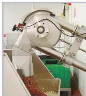
Interlocked inspection hatch in sprocket housing.
