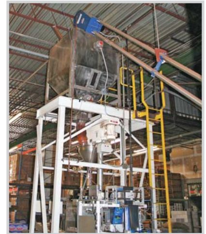
An AMC transferring flavoured coffee powder from a blender up to a packing machine.
