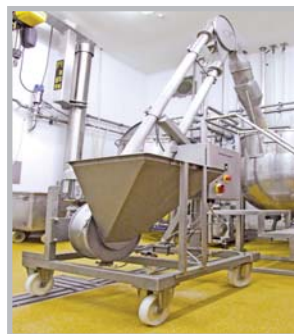
With simple sack tip hopper for non-dusty materials.
