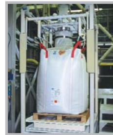
Automatic bag loop release.
