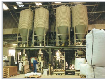
Filling materials in Bulk Bags and 25kg sacks in a minerals processing plant.
