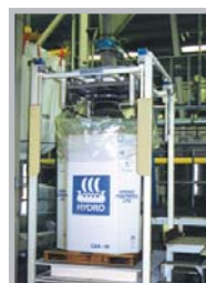
Using the same basic filling platform, special adaptors can be supplied to fill product in to other types of containers such as rigid IBCs, drums and tubs.
