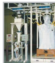
Using the same basic filling platform, special adaptors can be supplied to fill product in to other types of containers such as rigid IBCs, drums and tubs.
