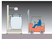
Series C fillers for handling bags on pallets.
