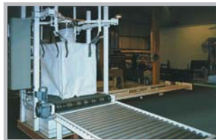
Using the same basic filling platform, special adaptors can be supplied to fill product in to other types of containers such as rigid IBCs, drums and tubs.
