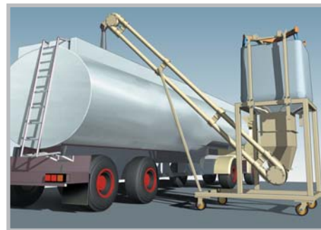
Aero mechanical conveyor mounted on a mobile frame loading road tankers.
