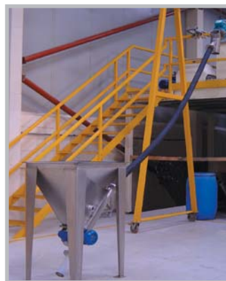
Our range of 'Rhinoveyor' Flexible Screw Conveyors are for very abrasive applications such as sand, cement, minerals and aggregates.
