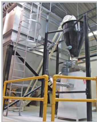
Aero mechanical conveyor elevating chemicals. Discharge heights can be specified for individual requirements.
