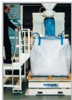
Optional equipment includes attachments for rigid bin and drum filling and a weight controller with data management.
