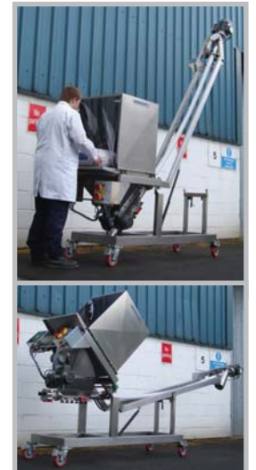
A single 'Spiroflow' mobile conveyor can be used to feed several items of equipment and/or can be removed to a dedicated wash-down area. Models are available with tilting booms for even easier cleaning or to negotiate areas of low headroom.
