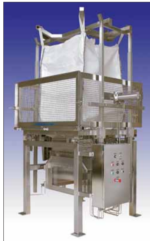
Spiroflow pharmaceutical-quality bulk bag discharger.
