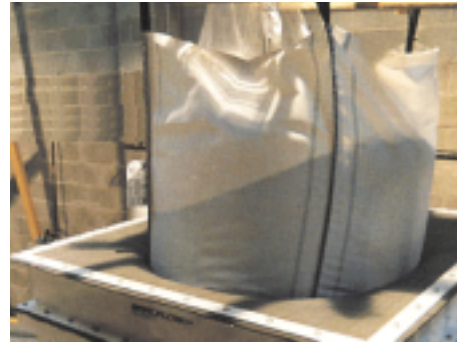
Secondary dust chamber for single trip bags.
