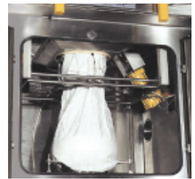
Inflatable spout sealing and stretching device (Patented)
