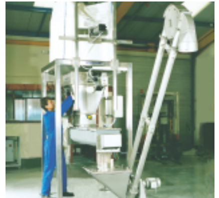
Aero mechanical conveyor
