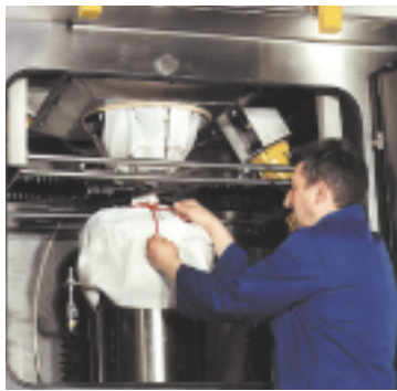
Spout closure bars close off bag whilst operator places spout over seal and unties the bag.
