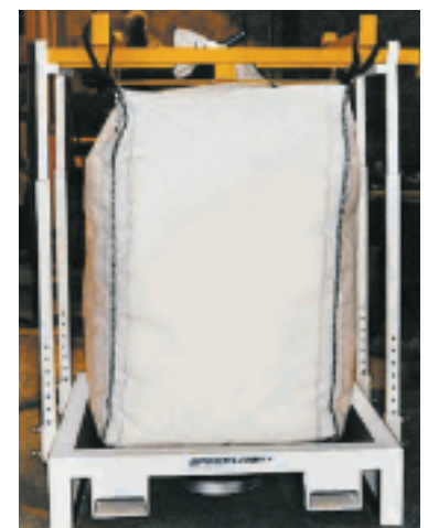
Low loading discharger with split top and base sections.
