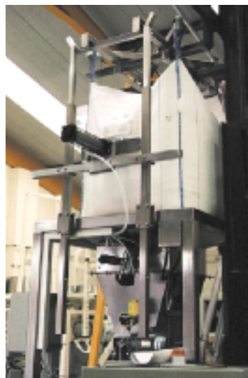
2. Bag is lifted by FLT on to discharger and kept under tension with spring loaded side support arms.
