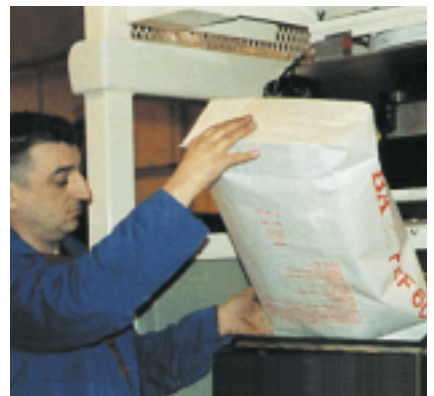
Sack tip door in discharger base.
