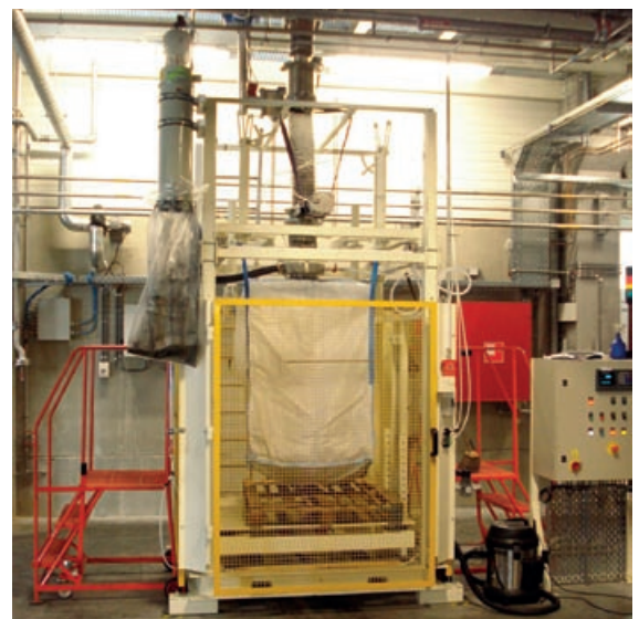
Filling by weight - hang weighing
