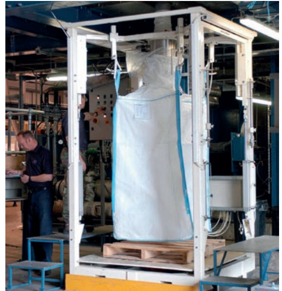
Filling by weight - platform mounted load cells
