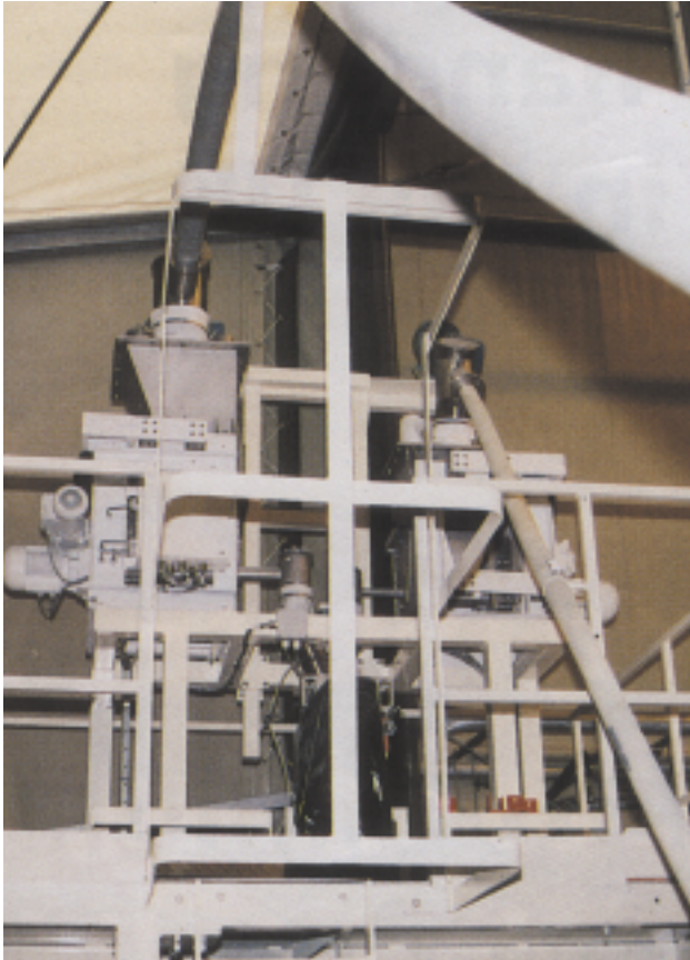
Ingredients are conveyed steeply from source to the process using flexible screw conveyors.
