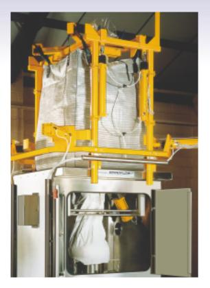
conductive and corona discharge, dispensing with the need to ground the bag. It employs hundreds of small patches, each with minute spikes which are not connected together. The low capacitance of the individual spikes ensures constant corona discharge, but at so low energy as to prevent ignition of combustible atmospheres.
