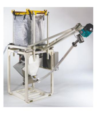
Couple this with the risk of powder being thrown into the atmosphere during the emptying process, and a brush discharge could cause the product or atmosphere to ignite resulting in a fire or an explosion.
