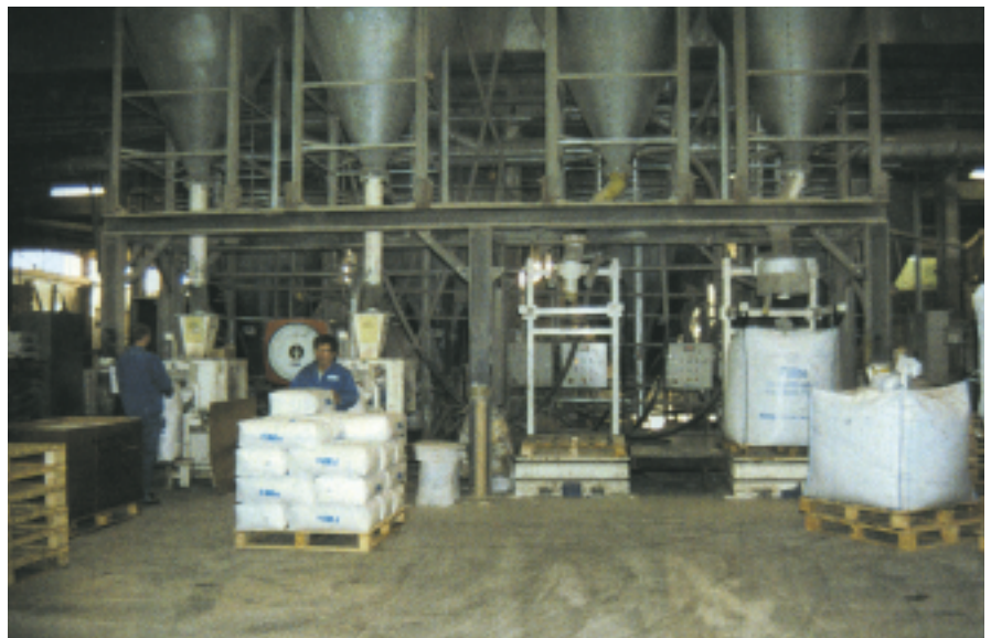
Impeller sack packer running alongside FIBC fillers at a cement factory
